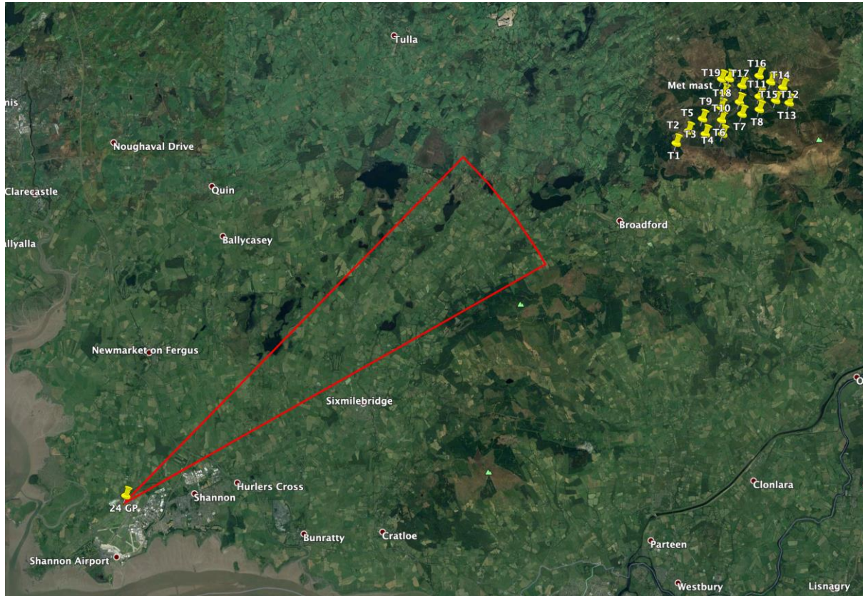
Figure 3.5 - Runway 24 ILS Glide Path Lateral Coverage Sector
