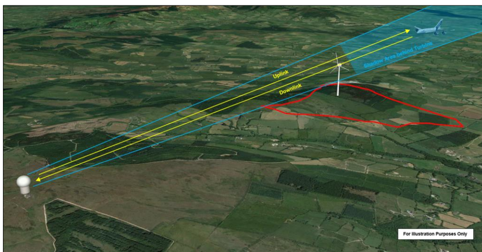
Figure 2. Shadow Area behind Wind Turbine
